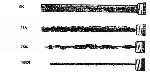
Replacement of the anode rod is recommended when consumption or weight loss is greater than 75%. The sacrificial anode equalizes aggressive water action providing cathodic protection for the tank. The anode is a very important factor in tank life and should only be removed for inspection or draining.
