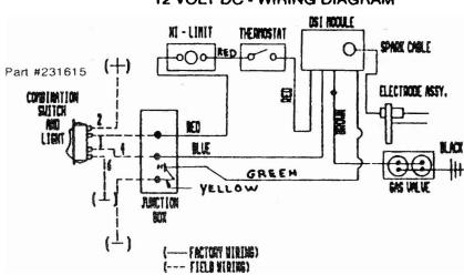
12 VOLT DC - WIRING DIAGRAM
