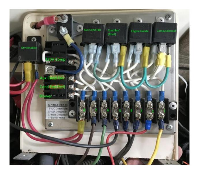
The basic layout based on the Starcool Panel, I have labeled the relays by their function, Below is the schematic with the same labels and more
